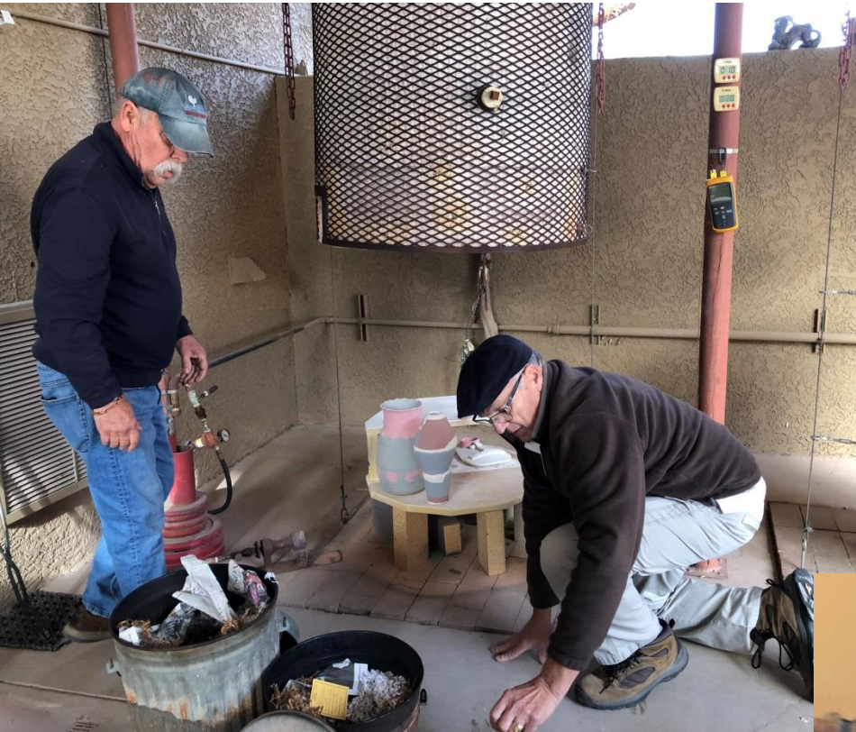
Step two: Load the gas fired kiln. Rob Altstaetter (L) and Doug Davis (R) load the pots out of the roasting pans onto the kiln shelves, keeping the roasters in line for later unloading. The pots need to fit just right.
